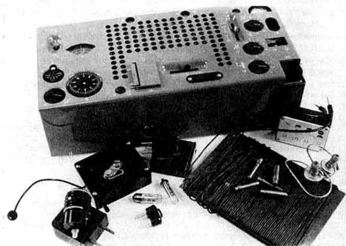
The British Mk123 transmitter-receiver with built-in mains psu which was originally developed about 1956 and which remained in service for paramilitary operations for nearly 20 years. Still provides a usable cw rig on 3.5/7/10/14MHz amateur bands. Shown here with some of the associated accessories including spare EF92/EF93 sub-miniature valves, mains-plug and crystal-holder adaptors, "reel" antenna as well as 100ft of antenna wire, neon-tester to indicate whether 110 or 220V mains, ac or dc. There is a built-in morse-key (right-hand bottom corner) but also a socket for use with an external manual or high-speed auto-keyer. Photo: Wendy Gilles, IBA
